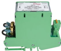
Example of a closed, toroid current clamp used (GF1).
