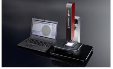
The PAMAS FastPatch 2 GO produces quick and accurate analytic results with the length, width and area of each particle recorded. The report of the microscopic analysis includes digital pictures of the membrane filtered samples according to ISO 4407. Results of the same sample are repeatable, regardless of the patch orientation or timescales between analyses.
