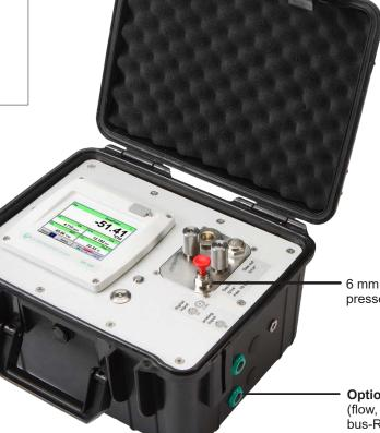
6 mm plug connection for measuring gas/compressed air feed
