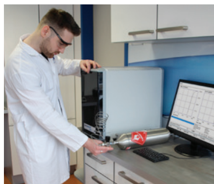
The Aquamax KF PRO LPG is designed for an easy and accurate determination of water in liquefied and gaseous samples such as LPG and LNG. The new device combines coulometric Karl Fischer method with a unique gasevaporation and dosing procedure.
